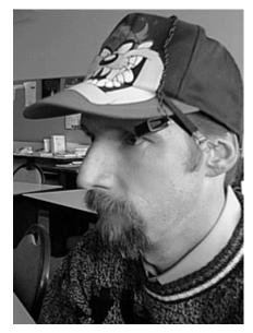
Here, the man blinks to interrupt an infrared beam. When the beam is broken, the switch closes.
