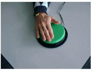
This person is using a switch that responds to pressure. By compressing the switch, they create switch actions.
