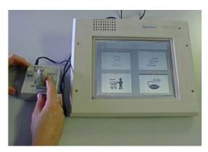
This multiple function switch, in contrast to the previous switch, has 5 possible on/off switches.
