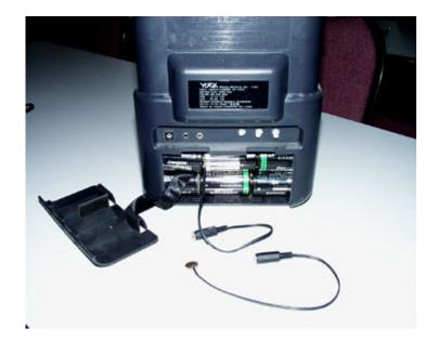
The switch is then connected to the interrupt and, voila', you have a fully accessible TV/radio that can be operated with the press of a hand (or any other body part) - see below.
