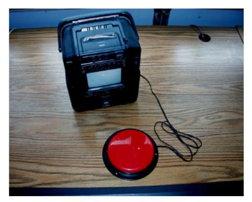
But what about AC (wall) current? Good question. You would not want to attach a switch to AC current without modification because this arrangement would send all 220 volts right through the switch. Chances are that the person would only have one opportunity to try out the switch before they were zapped. This would not be good. Fortunately, there
