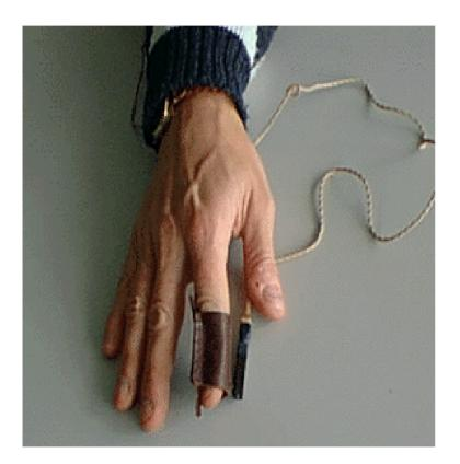
Wait for the finger to move (in slideshow mode) This handy switch is operated by bringing the two magnets together (one magnet is pictured below the finger and one is sewn inside the leather sleeve on the person's finger). This completes the electrical circuit and activates the device to which the switch is attached. Here the switch would activate a radio (not shown in the photo)
