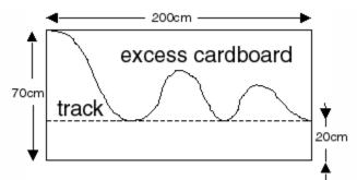
From the excess cardboard, students should cut out twenty-five  $4 \text{ cm} \times 12 \text{ cm}$  rectangles. These rectangles will serve as spacers between the two cutout tracks. Put glue along both of the 12-centimeter edges and fasten them to various places between the two tracks so that the tracks are rigid and separated by a distance of 4 centimeters.
